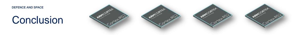
The DAHLIA H2020 project covers the development of a rad-hard high performance quad-core ARM R52 SoC in 28nm FDSOI technology, with eFPGA for flexibility and key IPs.
